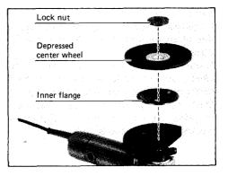
To tighten the lock nut, press the shaft lock firmly so that the spindle cannot revolve, then use the lock nut wrench and securely tighten clockwise.
